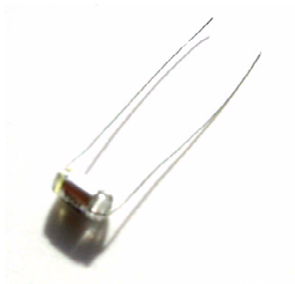
Figure 29: A 100\text{pF} PolyStrene Leaded Capacitor
