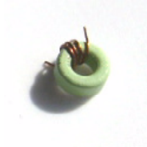
Figure 37: A 0.1\mu\text{H} T30-12 Iron Powder Toroidal Core Inductor
