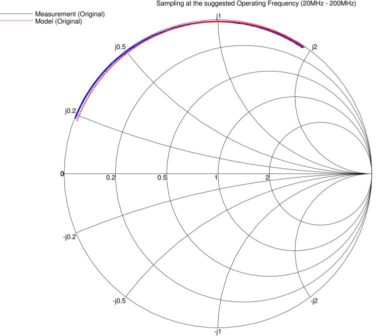
0.1uH Iron Powder Toroidal Core (T-30-12) Leaded Inductor with Wire Shortened Sampling at the suggested Operating Frequency (20MHz - 200MHz)
